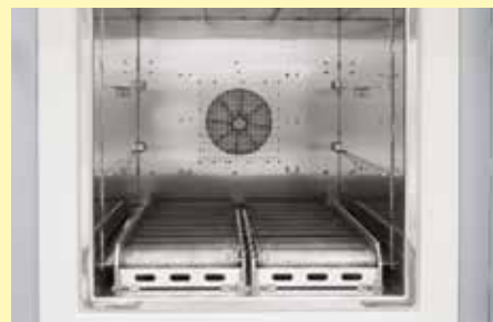
Roller conveyor in furnace chamber
