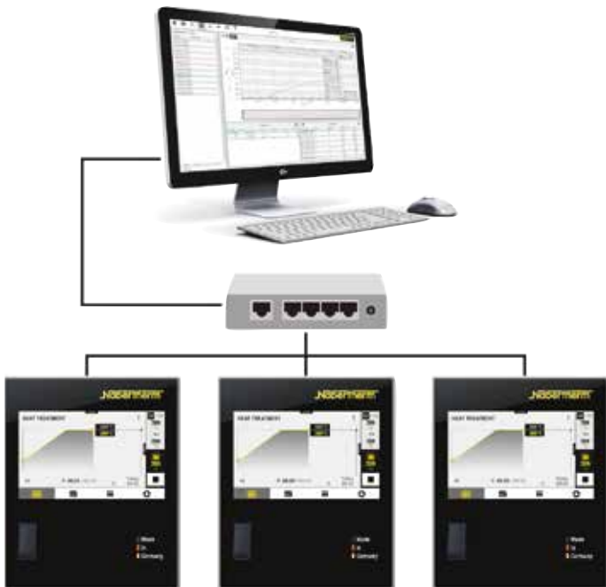
Example lay-out with 3 furnaces
