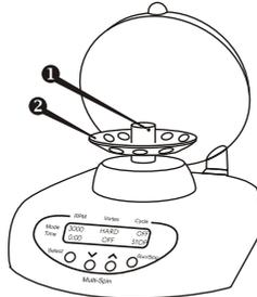
**Fig.1 Rotor replacement**
